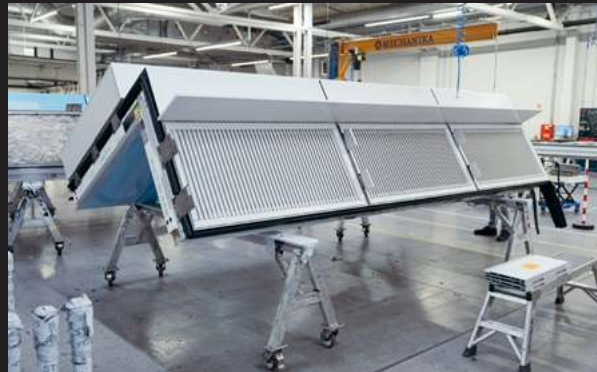
Production of façade elements for One Exchange
