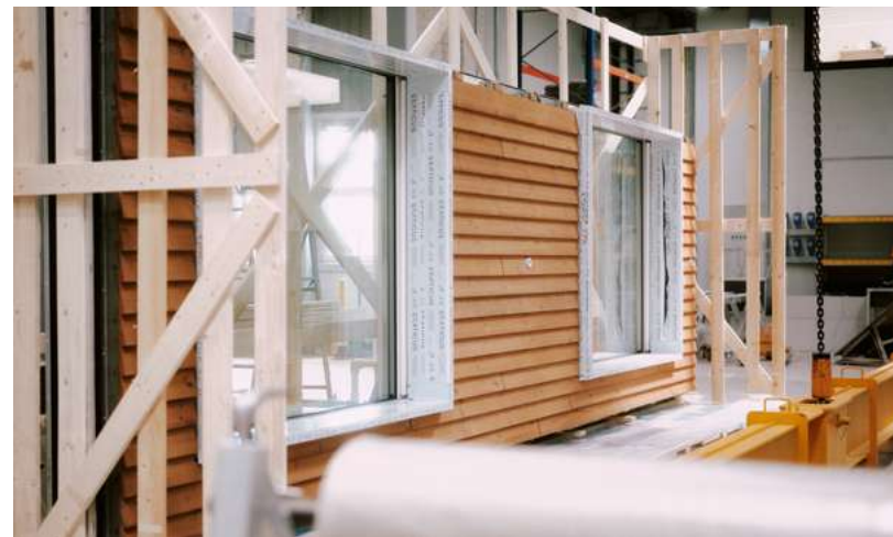
Wooden stillages designed for the transportation of façade elements from the factory to the construction site
