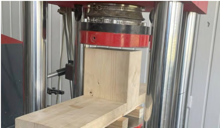
Testing frame connections for HUF
