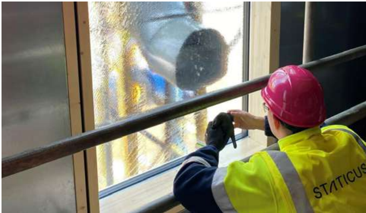
Testing the weathertightness of HUF
